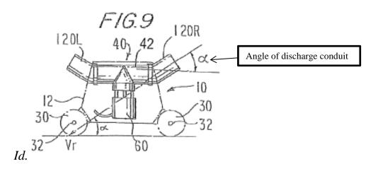
The water jet propels the cleaner to provide controlled random movement
