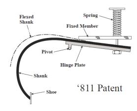
hinge plate upwards to urge the shoe into the ground but compressed to allow pivoting movement of the hinge plate about the pivot axis in response to the shoe hitting a rock. $^{113}$
