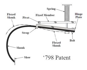
plate, ran through the stirrup (strap), and curved several feet down to the tiller shoe or plow. <sup>123</sup> In this combination of elements, the shank could flex and bow away from the bottom surface of the hinge plate (as shown in dashed lines) using the stirrup as a fulcrum between the oppositely bowed lengths of the shank. <sup>124</sup>
