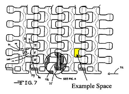
The Habasit patent describes, and the claims state, that the space between the link ends has a diameter of less than 10 mm when the belt is at its maximum extension, "to prevent fingers from penetrating the grid." '680 patent, col.1 l.60.
