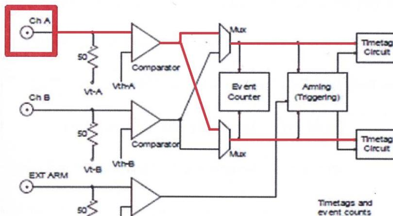
J.A. 1263 (color modified). In the above schematic, a user sets the circuit to One-Channel-Two Edge Mode with
